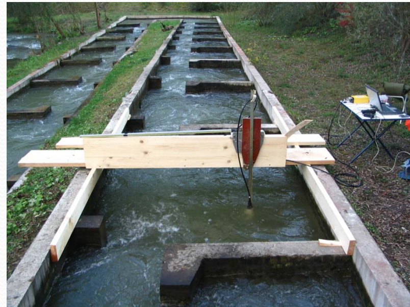
Velocity measurements with a 3D ADV probe
